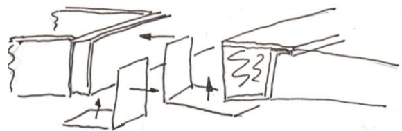
Icarex flap hinges applied to spar faces and spar bottom (or top for top hinge)
